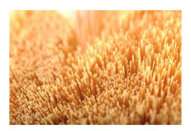
**Capture:** Efficient nitrogen separation using hollow-fiber membranes. In SEPURAN® N2 Evonik Industries has developed a new hollow-fiber membrane for efficient nitrogen production.
